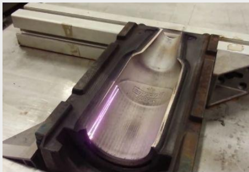
Mould Degrease Cleaning
