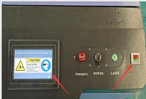
Air Pressure Alarm Device
